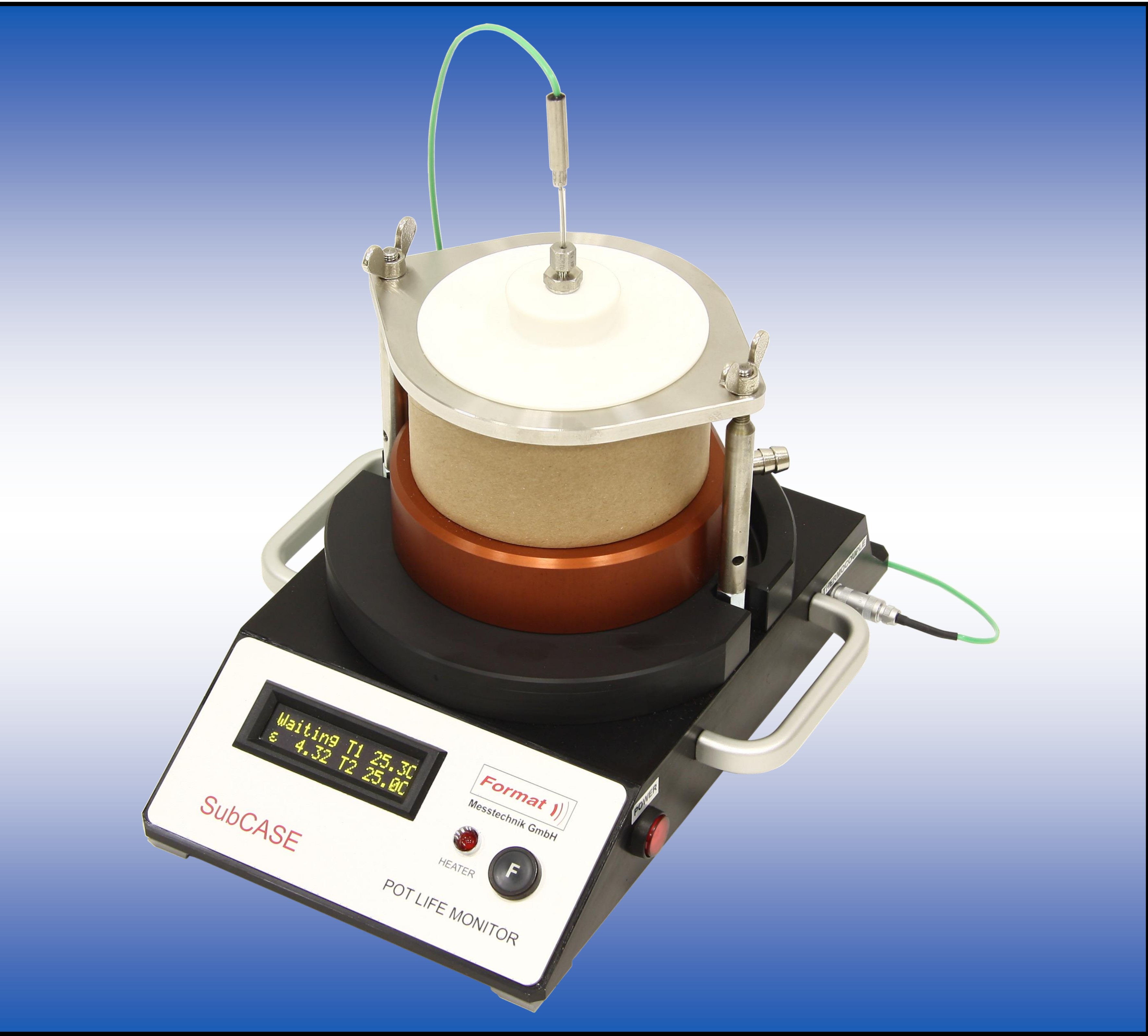
Fig. 1: The SubCASE® LT is designed to measure the gelling and curing reaction at low and constant temperatures. The relative permittivity of a formulation is measured simultaneously at different electric frequencies.
