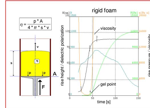
Fig. 5: The viscosity value is calculated by using the physical model of Hagen-Poiseuille, which is applied to a rigid foam measured with FOAMAT®. patent 19730891
