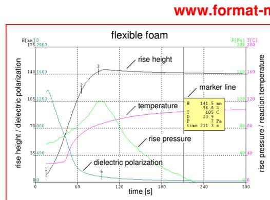
Fig. 2: The measurement data for rise height, temperature, rise pressure, and dielectric polarization is recorded simultaneously by the software FOAM and is displayed in one graph.
